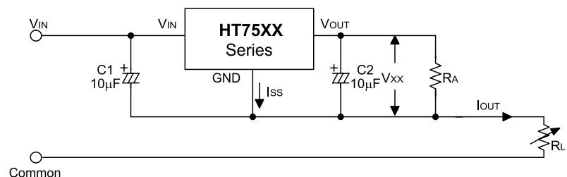
$$I_{OUT} = \frac{V_{xx}}{R_A} + I_{ss}$$
