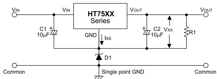
$$V_{OUT} = V_{xx} + V_{D1}$$
